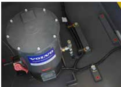
Auto lubrication system
