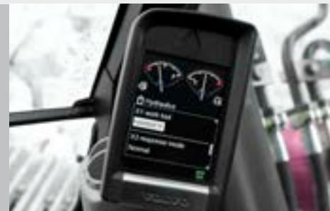
Hammer & shear: variable flow and pressure pre-setting
