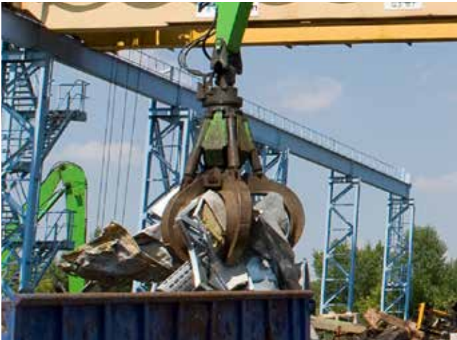
Orange peel grab (SGM), shell form half-open, e.g. for mixed scrap
