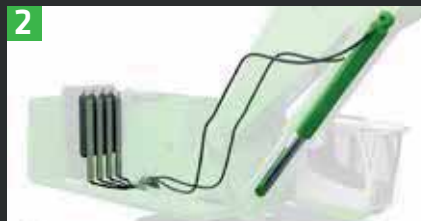
2 Energy storage module consisting of nitrogen piston accumulators
